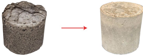
FIGURE 1: SAMPLES SHOW THE IMPACT BEFORE AND AFTER THESE CHANGES DESCRIBED IN THIS SECTION. BEFORE (LEFT) HAVING BUBBLY TOP AND VISIBLE PORES, AFTER (RIGHT) HAVING SMOOTHER EDGES AND FLAT TOP.
