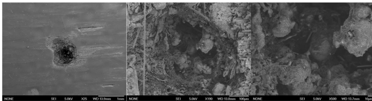
Figure 10. SEM images for Panel 3 at central region at different magnification levels.
